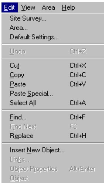
Use these menu items to edit an open Spectrum24 site survey, display a list of coverage areas within the workspace and use the **Setup**, **Meter Settings**, **Sounds** and **Logging** property pages to configure surveyor, system sounds and test data logging information. Use the menu items below **Default Settings** to edit the report file.
