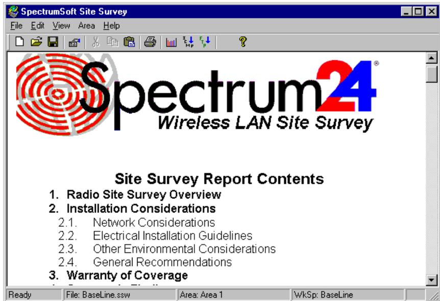
The report is a Microsoft WordPad document that can be generated when the survey is complete. The report can be edited and printed using the Cut, Copy, Paste and Print application toolbar buttons. The template for a new report has a Site Survey Results.doc filename and is installed in the same directory as the program executable.
