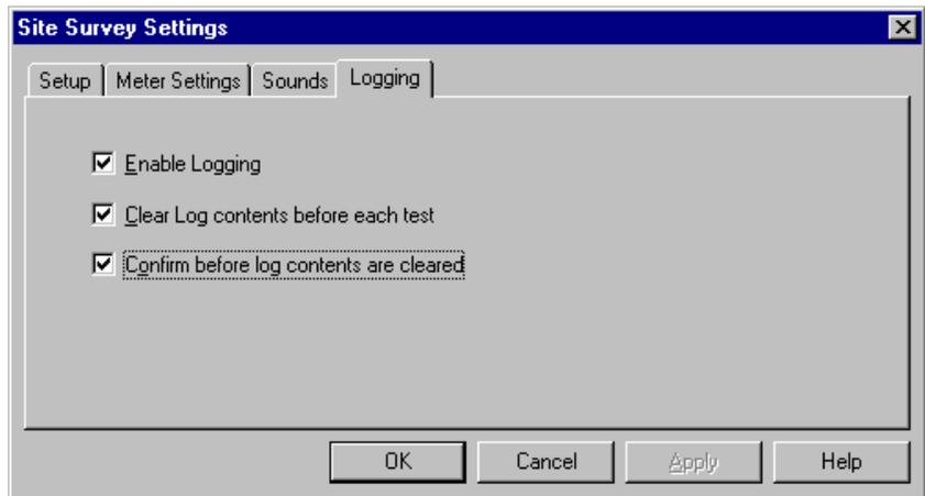
**Clear Log contents before each test.** Select **Clear Log contents before each test** to automatically clear the content of the log before a test suite is run.
