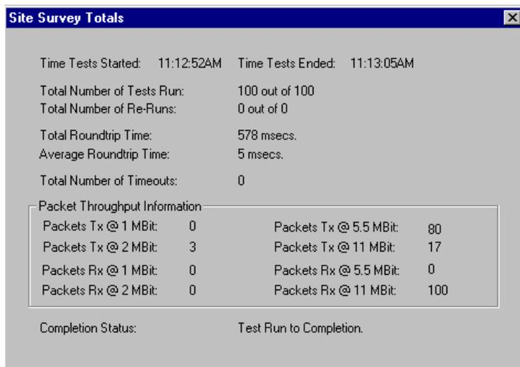
Use the **Site Survey Totals** dialog box to display the time the tests were started and stopped, the number of tests run, number of re-runs, total roundtrip time, average roundtrip time, total number of timeouts and the test completion status. Packet throughput information is summarized as the number of packets sent and received and the data rates for each. These values are recorded in the logfile if logging is enabled.
