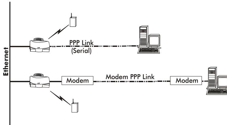
A PPP link provides the option of using a direct serial link or modem to extend wired Ethernet topologies.
