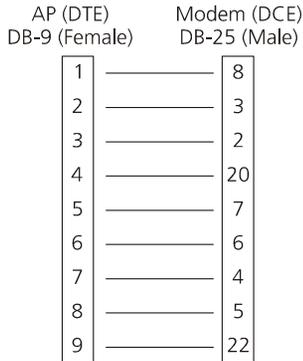
When using a modem connection, one access point represents the originating access point and the other represents the answering access point. When using a PPP link, do not use the serial port to access the UI. Access to the UI requires establishing a Telnet session with the access point.
