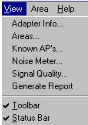
Use the menu items to view Spectrum24 WLAN adapter driver and Firmware data, site survey areas, access points within range of a target Spectrum24 mobile device and a graph depicting MU signal quality and to append the logfile to the report file. The status bar at the bottom of the main window can be displayed or hidden by checking or unchecking **Status Bar**. The tool bar buttons can be displayed or hidden by checking or unchecking **Toolbar**.
