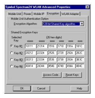
Use the Encryption Algorithm pull-down menu to select the Open System, 40-bit or 128-bit Encryption algorithm to be used for the adapter. The Open System algorithm (default setting) does not encrypt packets over the network. Select Open System to disable Encryption for the WLAN adapter and allow for the transmission and receipt of data with no security.
