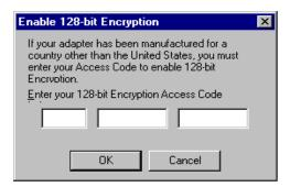
Once 128-bit Encryption is enabled, select 128-bit Encryption from the Encryption Algorithm pull-down menu. Enter the 26 Hex digit Encryption key by spreading the 26 Hex digits across the six fields provided. Click OK to save and implement the Encryption key data.
