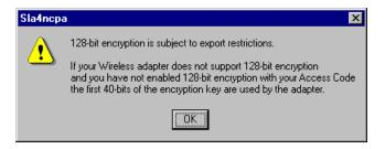
If an access code is required, click the Access Code button to display the Enable 128-bit Encryption dialog box. Enter the access code in the three fields provided and click OK. Once the access code is entered, the Access Code button is no longer displayed on the Encryption property page and the access code is stored.
