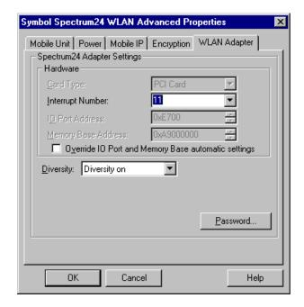
Select Diversity if dual antenna support is required. Diversity improves communication in highly reflective environments. Do not select diversity if a secondary antenna is not being used. Using diversity in a single antenna application can cause poor wireless network performance.
