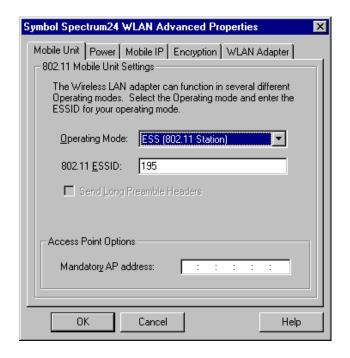
ESS (802.11 Station) - Select ESS (802.11 Station) to enable the MU to transmit and receive data with an access point. ESS is the MU default mode.
