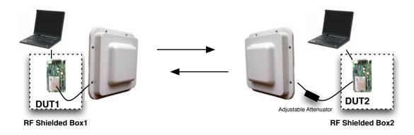
**TestSetup:** A few different 5GHz mini-PCI cards were tested against XR5 using a modeled range performance study. Under the same setup conditions, a pair of each card type was used in combination with Mikrotik RB112 boards and a link was established. Using the adjustable attenuator, path loss was introduced into the link and steadily increased until the link was lost. To prevent PCB coupling, each DUT was placed in a RF shielded box.
