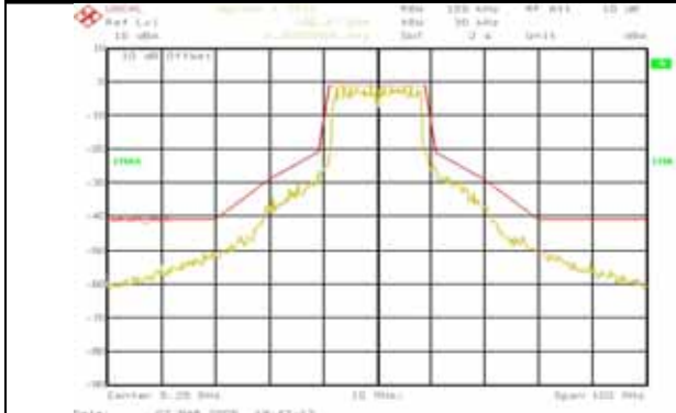
Typical OFDM Output Spectrum at Pout=+25dBm, 5.25GHz (Vc=5.0V, Icq=250mA, 64QAM / 54Mbps)
